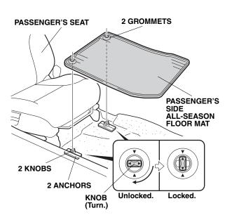
4. Place the grommets in the rear all-season floor mat over the anchors, and turn the knobs one quarter turn to secure the all-season floor mat.
