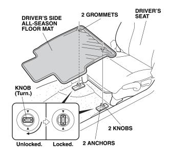
2. Place the grommets in the driver's side all-season floor mat over the anchors, and turn the knobs one quarter turn to secure the all-season floor mat.
